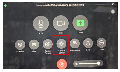
4. On the control page, you can control the camera's PTZ movement and activate its tracking function by pressing the Presenter Focus button.
